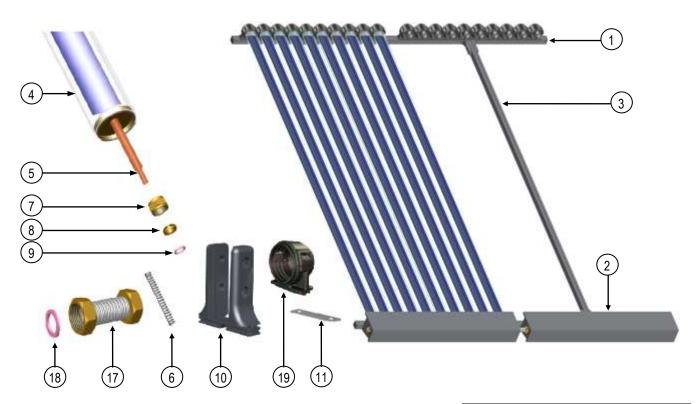
Preparation of the vacuum tube to be encased in the KSR10 solar collector
